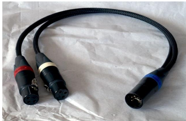
X5-IN, XLR-5M to 2x XLR-3F audio signal cable, Length 0.3m provides an input to the power stages of the Isis on two standard 3-pin XLR female connectors
